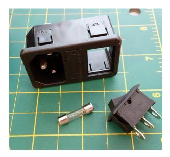
1. Install the switch into the IEC. Note the orientation of the switch, steps 3 and 4 depend on it.
