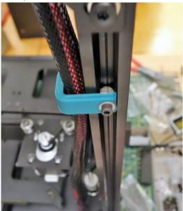
7. Cut a ~55cm long piece of the wire loom, and use it on the X motor and endstop wires.
