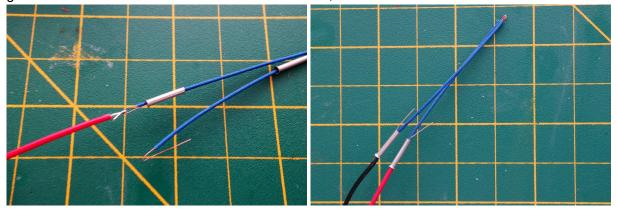
10. Make sure the fiberglass insulation is flush with the thermistor glass bead, and no lead is exposed. Using a crimping tool, or pliers, crimp the ferules.
