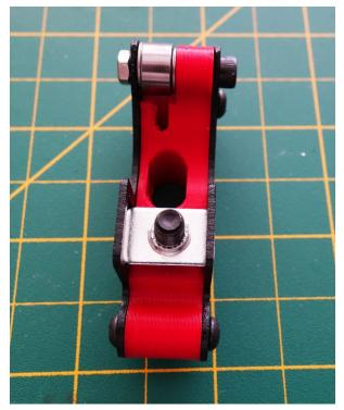
7. Install the completed lever arm to the extruder body with a M3×30 SHCS screw using a washer next to the screw head. Use thread lock on this screw. Tighten but leave loose enough so the lever arm can move. Do not install the brass hob yet.
