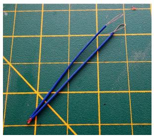
7. Slide the ferrules on the leads, and bend the exposed leads as shown.
