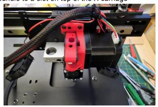
5. Insert the other side of the bundle, into a cutout on the left side of the Top Deck Left, by the Z extrusion.
