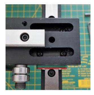
3. Mount the left side (when the printer is upright that will be the right side) using four M3 × 10 SHCS, 8 M3 Washer, and four O-Rings. Assemble in the following order: M3 × 10 SHCS > M3 Washer > O-Ring > M3 Washer > X Axis plate. Leave the screws slightly loose.
