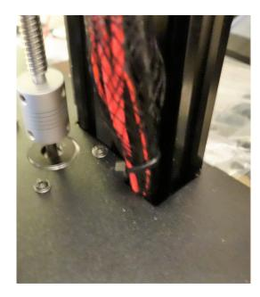
6. Using a M3 Post Install Nut, a M3 × 10 SHCS, and a printed clip, secure the bundle to the back of the left Z extrusion, about 2" from the top.
