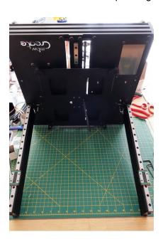
2. Mount the right end (when the printer is upright that will be the left end) of the X axis to the Z rails using **four M3 × 6 BHCS without washers.** Leave the screws just slightly loose.
