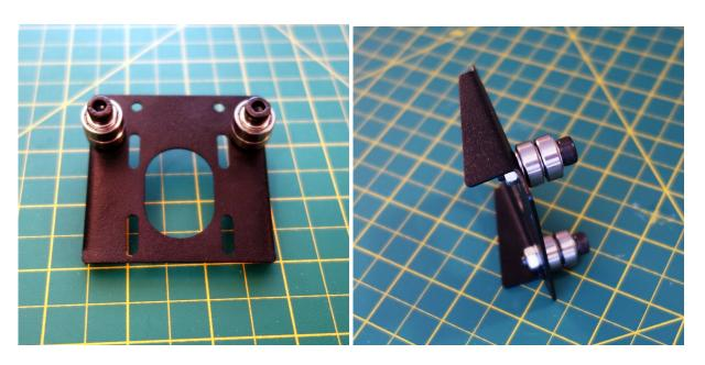
New Create kits are provided with a vibration dampening mount for this axis. Two of the holes on the mount are not tapped. Use these holes and two m3-6 button head screws to attach the mount to the stepper motor.
