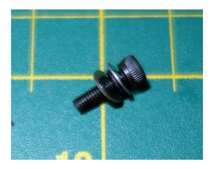
The O-Rings here help allow for any slight misalignment, guaranteeing smooth, bind-free movement.
