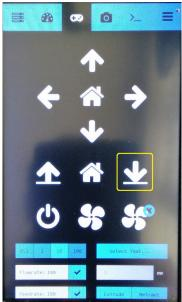
7. We are now going to raise the Z by pressing the **Arrow up** button and count each time you press the button until the LED on the sensor goes off.
