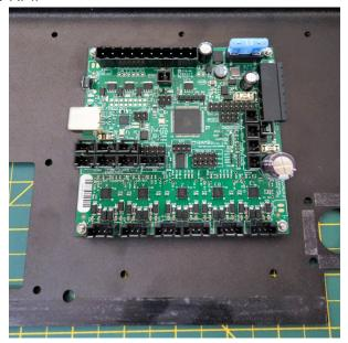
Tighten the nuts holding the RAMBo Controller, carefully so not to damage any of the board components.
