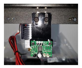
3. Connect the sensor wire. Note the orientation of the connector, the **green** wire should be on the **OUT** pin, and the **red** wire on the **VCC** pin.
