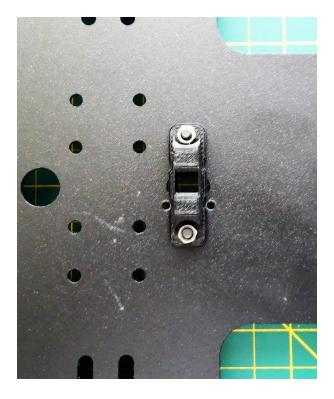
4. Mount the Y Carriage Plate onto the Y Axis Assembly, using 4 M3 × 6 BHCS and four M3 Washer.
