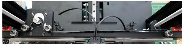
5. Push on one side of the **X Belt Clip** to hold the belt. Pull on the other side to tension.
