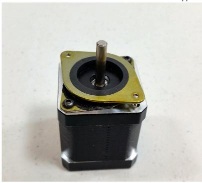
1. Install the Y Motor assembly with 2 M3 × 6 BHCS and 2 M3 Washer. These screws will insert into the tapped holes of the vibration dampening mount. See the pictures below for the proper orientation relative to the rest of the assembly. Be sure that the motor is in the uppermost position so when we later install the belt you have plenty of room to adjust it.
