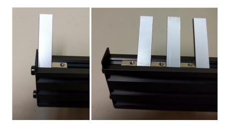
Be sure all the nuts are inserted in the same orientation or the spacing will be incorrect. For easiest insertion, insert the end with the spring ball into the slot first as shown below
