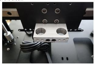
3. Install the <u>printed extruder body</u> to the carriage with **two M3 × 6 BHCS** screws. Also attach it to the Hotend Block with a **M3×18 SHCS**
