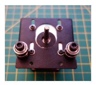
3. Install the pulley, leaving about 1-2mm between the bottom of the pulley and the top of the motor mount plaTE. Install it with the set screw end of the pulley toward the motor (The opposite of how it pictured). Be sure one of the pulley set screws is aligned with the flat of the motor shaft.
