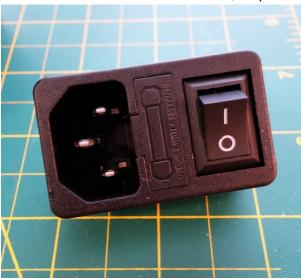
2. Install the fuse into the IEC
