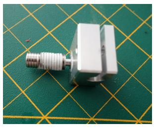
3. Install the heatblock assembly into the heatsink, tighten it slightly using the supplied wrench. Do not over tighten, that can damage the heatbreak.
