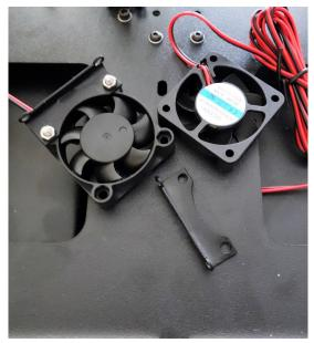
2. Install the Fan Mount on the X Carriage Plate as shown. Repeat on the other side.
