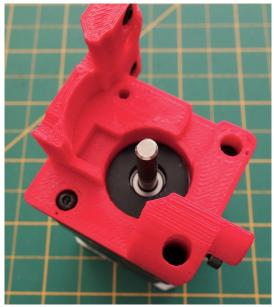
2. Attach the Extruder Arm Plate with one M3 × 6 BHCS or a self tapping screw to the right side of the printed piece
