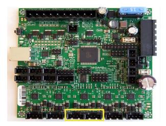
4. Attach the (Default) Right Extruder Stepper to the RAMBo E0 Driver plug, the blue goes toward the USB Port. If you are installing a second Extruder Stepper to E1 Driver plug, install the second extruder plug reversed. This makes the motor run in reverse, which is needed since the second extruder is a mirror image of the first.
