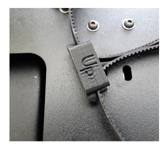
2. Install the X Belt Spacer on the X Carriage Plate with two M3 × 6 BHCS
