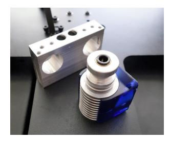
2. Install the <u>Aluminum hot end block</u> to the carriage with **two M3 × 10 SHCS** inserted into the deep holes that are center front of the block.
