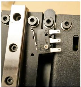
5. The endstop wires are provided with the RAMBo board, they are black and white, with spade connectors on one end, and a keyed connector on the other end. Connect them to the switch outside
