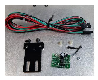
1. Attach the sensor to the acrylic mount using two M2 × 12 SHCS, two M2 Nuts, and the mini standoffs between the plate and the board as shown above.
