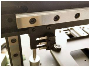
3. Install a M3 × 10 SHCS into the tapped hole on the X Carriage Plate as shown below
