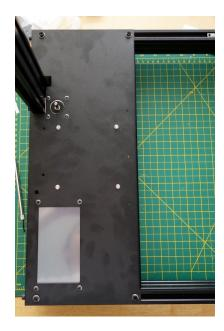
3. Align the assembly with the left edge of the base, so the motor is touching the vertical upright and tighten the plate, then the motor.
