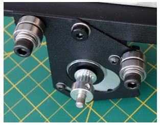
3. All three Idlers will Install in the following order: M5 × 20 SHCS > Zero or more M5 Washer as needed > 605zz Bearing > M5 Washer > 605zz Bearing > M5 Washer > Y Motor Mount or Machined Y Plate. The two upper idlers will screw directly into the tapped holes on the Machined Y Plate. The lower idle will screw into an M5 Nut Use as many washers below the screw head as needed to keep the bearings snugly in place (probably 2-3).
