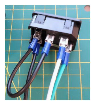
5. Insert the IEC with the wires into the IEC plate on the right side of the printer.
