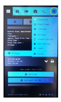
3. Click on the **Connection**. In the popup shown below check the Auto-connect box, press the **Connect** button, then close it with the **X** button.
