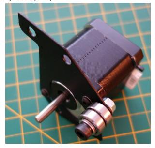
4. Locate the two 5mm tapped holes on the side of the Machined Y Plate and attach the Y motor plate using an Idler Bearing assembly and an M5 × 10 SHCS with a M5 Washer. See the images below for clarification.
