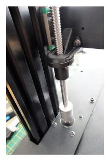
6. Tighten the set screws on the Helical Coupler.
