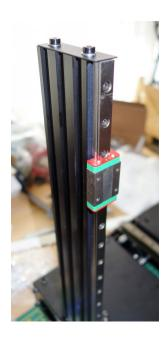
4. Tighten the screws holding the rails.
