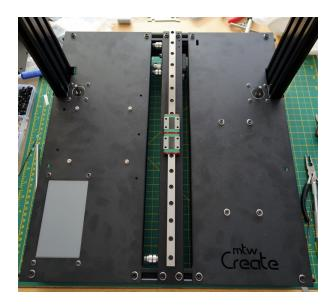
3. Align the assembly with the right edge of the base, so the motor is touching the vertical upright and tighten the plate, then the motor.
