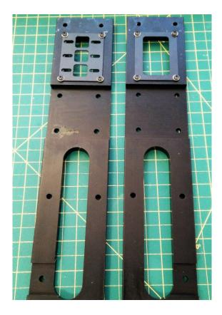
3. Loosely assemble the side plates to the 400mm extrusions using 8 M5  $\times$  16 SHCSs and 8 M5 Washers. Do not tighten the screws yet.
