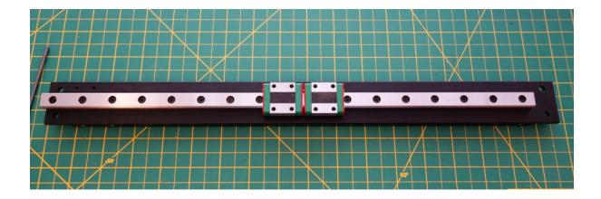
5. We recommend adding **one each M5 × 10 SHCS**, **M5 Washer** and **M5 Nut** temporarily to each end to each end of the assembly to prevent the cars from being able to come off.
